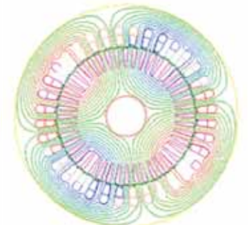
Equivalent fluxline of an induction motor
